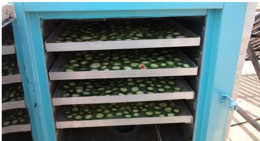
Figure – 2 Drying of Bitter Gourd in the Cabinet Dryer
